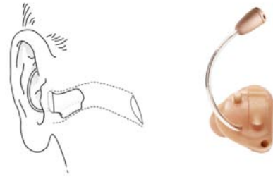
Figure 1: The placement of the microphone in the concha cymba hides the microphone not only for improved cosmetics but also for improved acoustic performance due to pinna effects.
